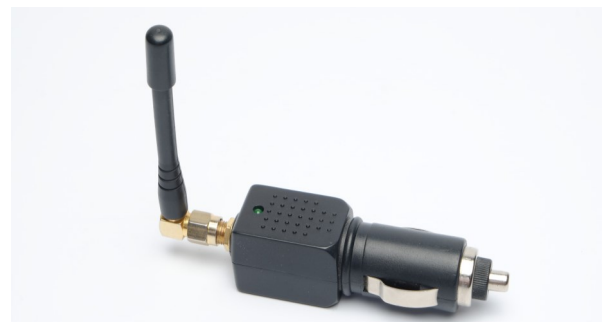
Typical cigarette lighter GPS jammer readily available on the Internet
