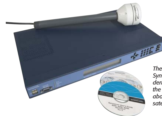
Above: Symmetricom’s SSU 2000, an intelligent, fully manageable Synchronisation Supply Unit or Timing Signal Generator Left: Detail of the SSU 2000
