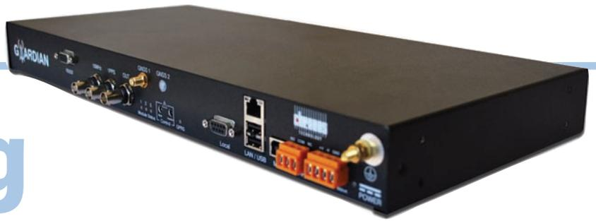
▲ 17 GAARDIAN units are currently deployed around the UK for measuring GNSS quality of service
