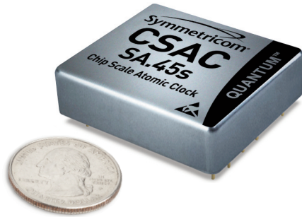
FIG 2 At only 16cm 3 , and with <115mW of power consumption, the SA.45s CSAC brings the benefits of an atomic clock to portable applications for the first time.
