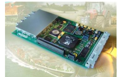
The PolaRx2 receiver is capable of providing accuracies from 1.2-2m down to 2-5cm, depending on the technique that is used. Special firmware is used to limit the influence of reflections and to re-acquire the GPS signals very fast after signal interruptions. This last feature is important as the straddle carriers are often moving beneath the large cranes, where GPS signals are sometimes obstructed.
