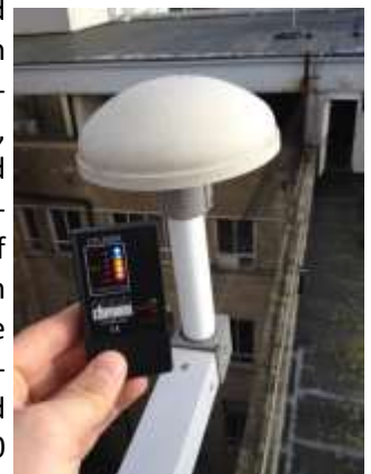
CTL3500 handheld GPS jamming detector
