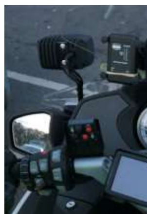
Close up of Jamming Detector on Motorbike
