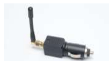
Typical cigarette lighter GPS jammer readily available on the Internet
