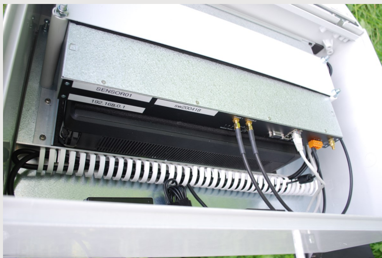
Probe deployed during outdoor GPS Jamming trials in IP65 weather-proof enclosure
