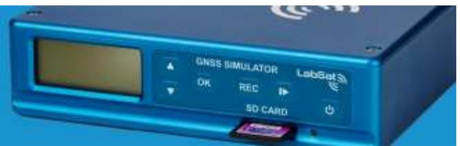
**LabSat 3** is a standalone, triple constellation simulator for testing devices based on satellite navigation systems; it is capable of recording and replaying multiple raw satellite navigation RF signals including GPS, GLONASS, Galileo, BeiDou, QZSS and SBAS. The optional SatGen software package can be used to generate simulated satellite signals from a user defined trajectory, allowing tests to be carried out simulating any time, date or place around the world.
