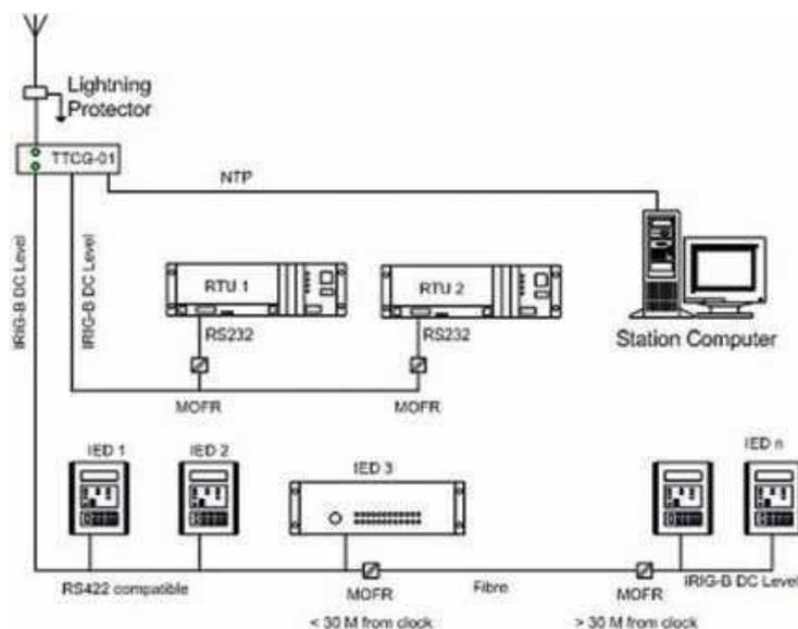
In the diagram we can see that IEDs in close proximity to the clock are cabled in shielded copper while those a greater distance away from the clock make use of fibre. Electrically harsh situations such as feeder protection relays being located close to the CB would also have the time sync distributed by fibre even when the distances are less than 30 metres.
